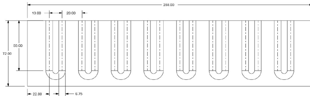
**Figure 5. Dimensions of the radiant "U-Tube" burners installed for 500 kW power.**
