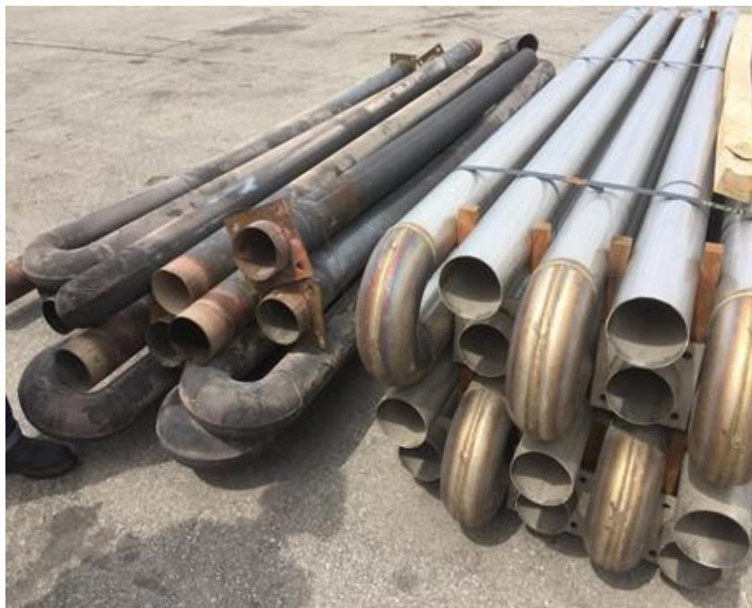
**Figure 4. Radiant tubes used in homogenization furnaces.**
