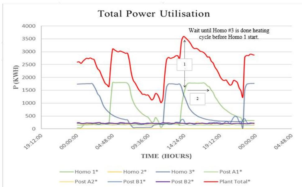
Figure 3. Foundry power utilization for all equipment on 1 December 2016.
