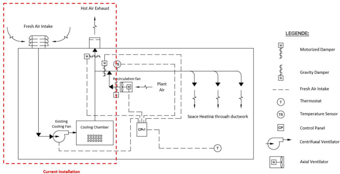
**Figure 6. Process Flow Diagram of the current and intended heating system.**
