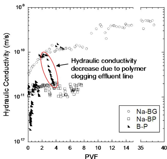
**Figure 2. Hydraulic conductivity vs. pore volumes of flow for Na-BG, Na-BP, and B-P GCLs permeated with bauxite liquor.**
