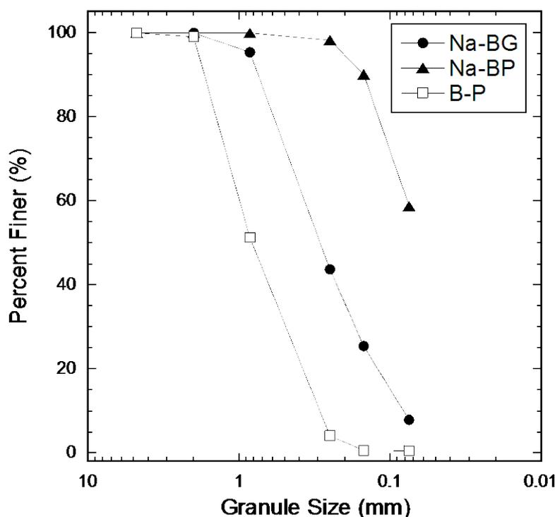
Figure 1. Granule size distributions of bentonites in GCLs used in this study.
