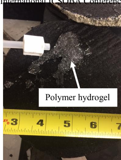
**Figure 3. Removing polymer hydrogel clogging the effluent tube.**
