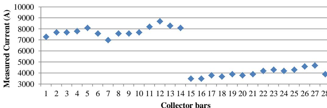
Figure 5. Cathode current distribution, pot 261, after 2 days.
