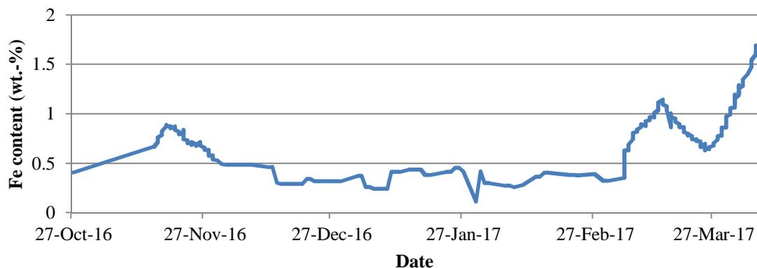
Figure 8. Fe Content of metal samples in wt.-%, pot 122.
