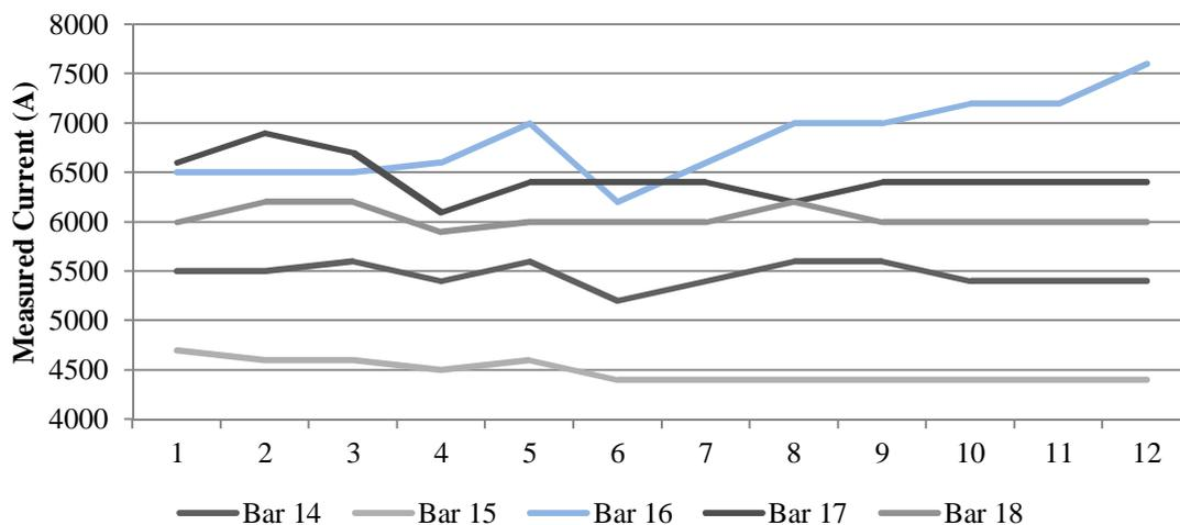
Figure 4. Cathode current distribution for pot 178, 12 measurements.
