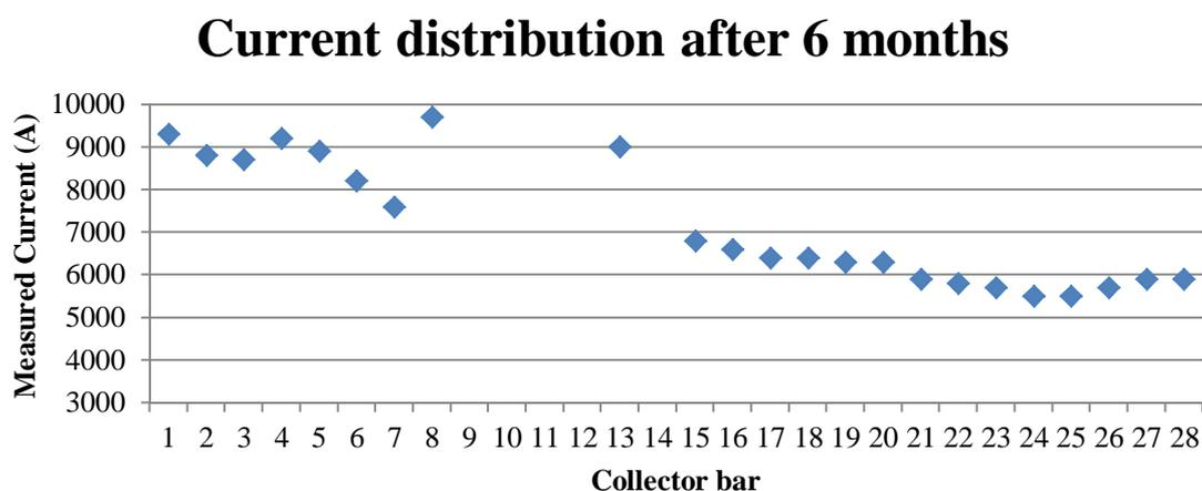
Figure 7. Cathode current distribution, Pot 261, after 6 months.
