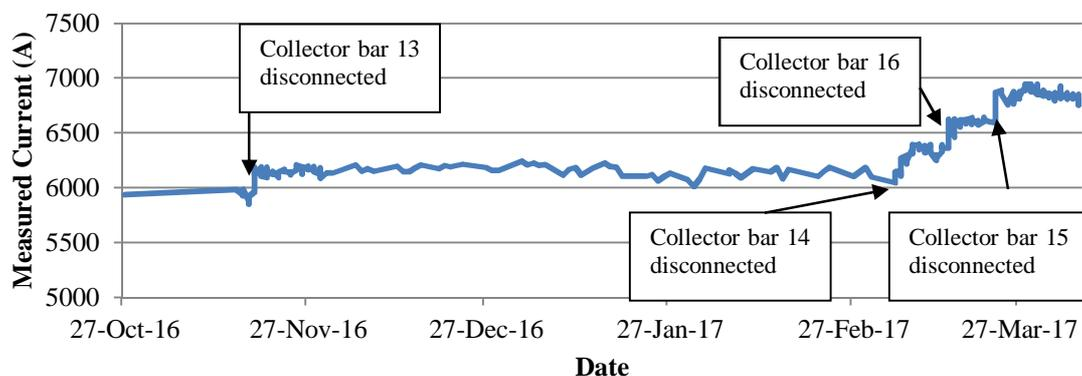
Figure 9. Average current in collector bars, Pot 122.
