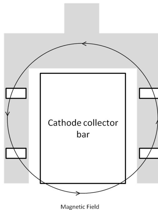
**Figure 2. Schematic of measuring tool with 4 hall sensors. Rectangles on the side are Hall sensors.**
