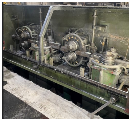
Figure 3. Reduction and calibration rolls of CRE line.
