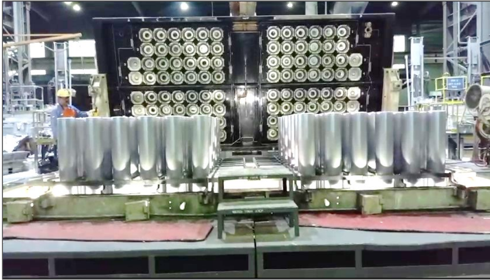
Figure 1. Air-slip casting table with mould and billets.
