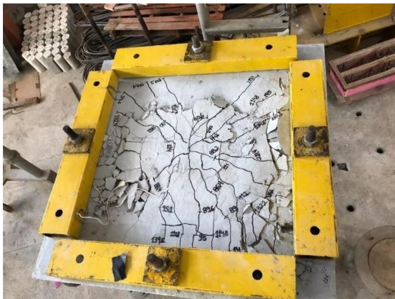
Figure 6. Puncture resistance test.
