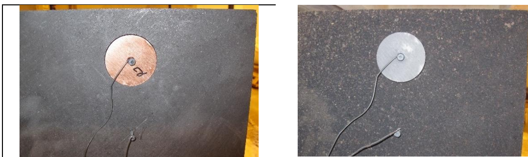
Figure 2. Initial crack testing. Left: before testing. Right: after testing, no visible cracks.
