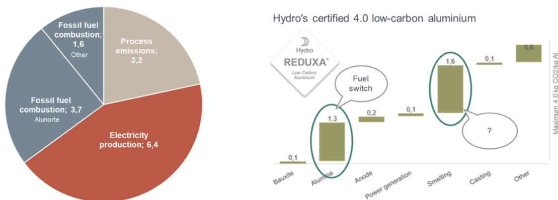
**Figure 1. CO<sub>2</sub> emissions in Norsk Hydro. Left: Hydro's total emissions sorted on source. Right: Emissions from the various steps in the value chain for the certified Reduxa low-carbon aluminium.**
