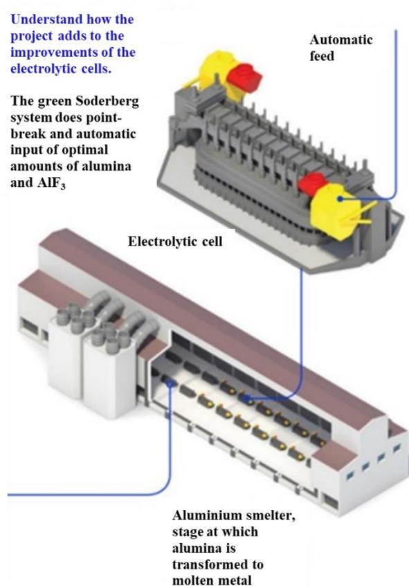
Figure 1. Schematic drawing of the point feeder pots.
