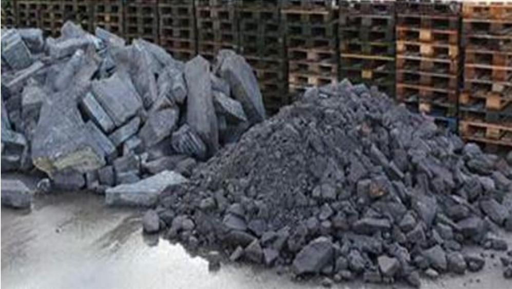
**Figure 1. SPL removed from the reduction cell.**
