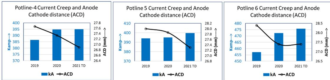
**Figure 1. Potline current increase (creep) and ACD.**
