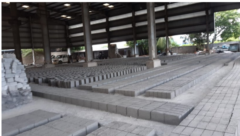
Figure 4. Bricks Produced Locally in Vizag with Lime Byproduct.
