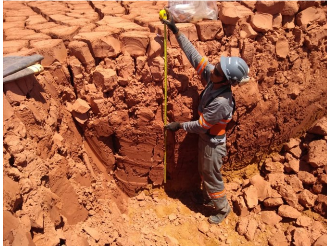
Figure 6. Excavated profile showing high tailings solids content.
