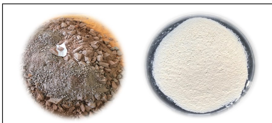
Raw PLK - 18% Fe 2 O 3 Chemically treated PLK ≤ 2% Fe 2 O 3 Figure 5. PLK before and after beneficiation.
