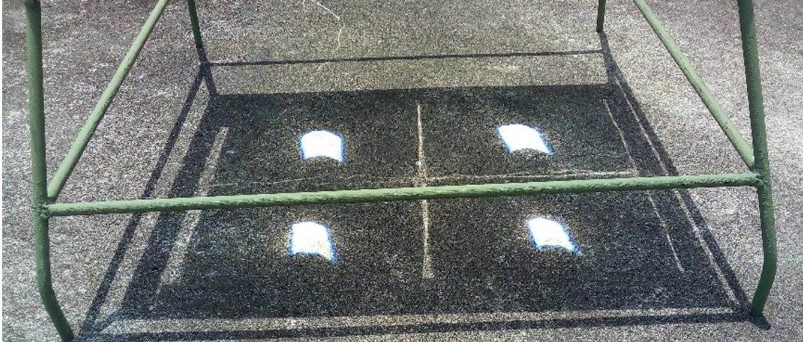
Figure 10. Four focus point Fresnel lens used to focus CSE onto ore being transported by conveyor belt.
