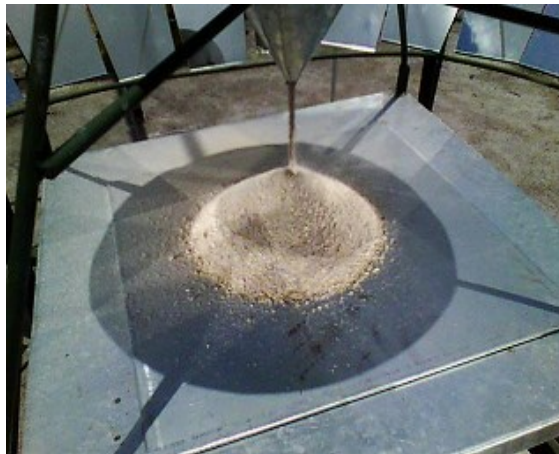
Figure 1. Experiment 1 set up showing the heliostats, funnel and sand dropping being hit by CSE from all sides. (Flir E4 model thermal camera – Normal mode)
