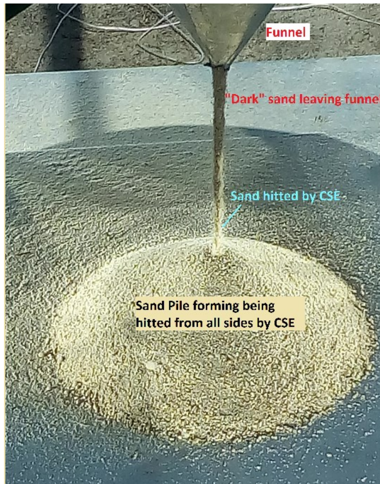
Figure 7. Detail of CSE hitting sand falling down from funnel.
