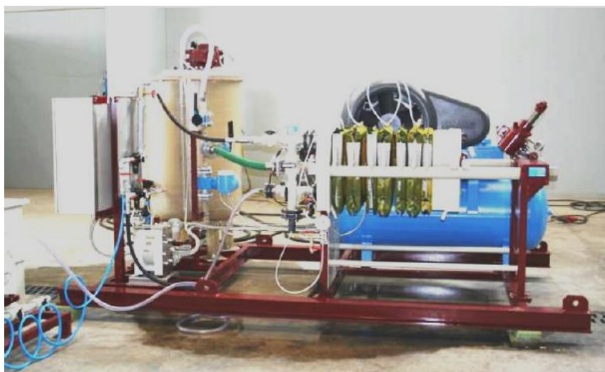
Figure 2. Pilot filter press unit.
