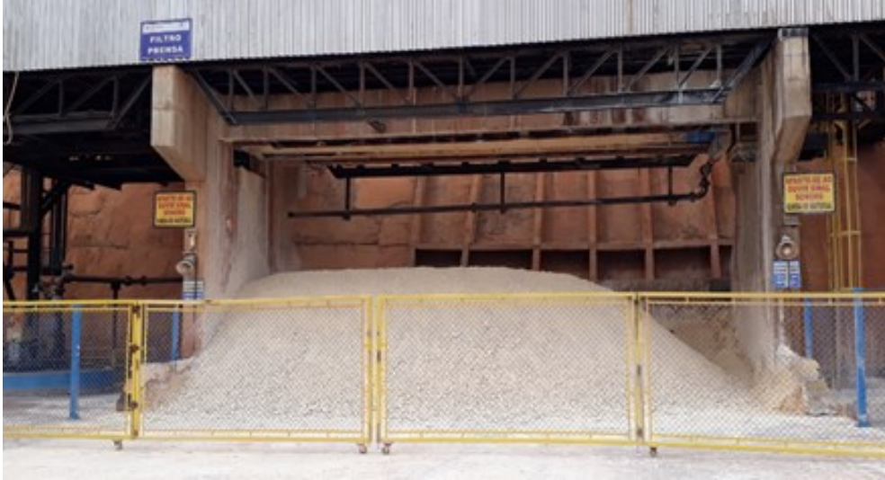
Figure 20. 10 t/h filter press discharge and calcium carbonate cake.
