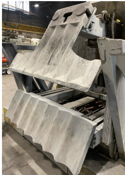
Figure 4. In-furnace dross processing skim and cold plate.
