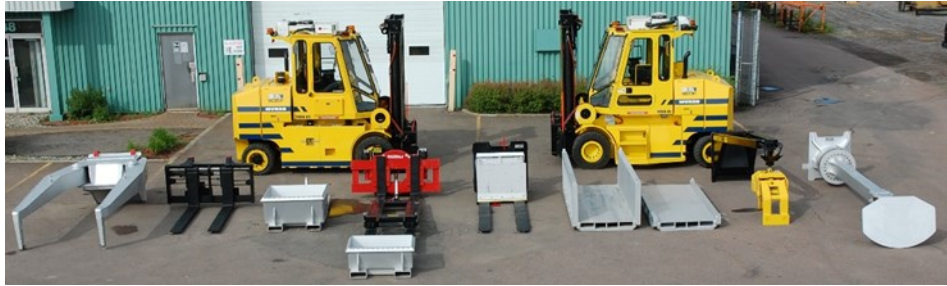
Figure 2. Mecfor Multipurpose Vehicle Casthouse solution - MVR and tools.
