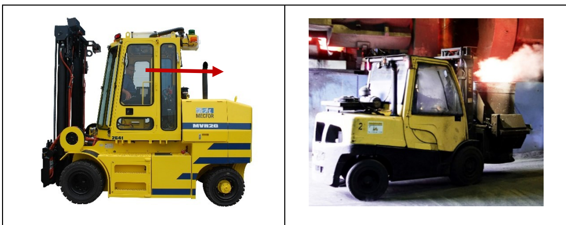
Figure 5. Left - MVR22 with rotating seat for optimal vision, facing forward, while driving. Right – Industrial forklift carrying a molten metal ladle.
