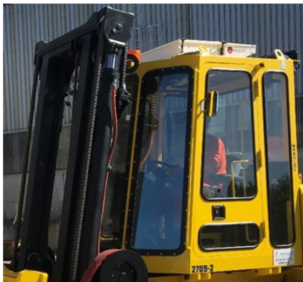
Figure 3. Special glass assembly for better protection.
