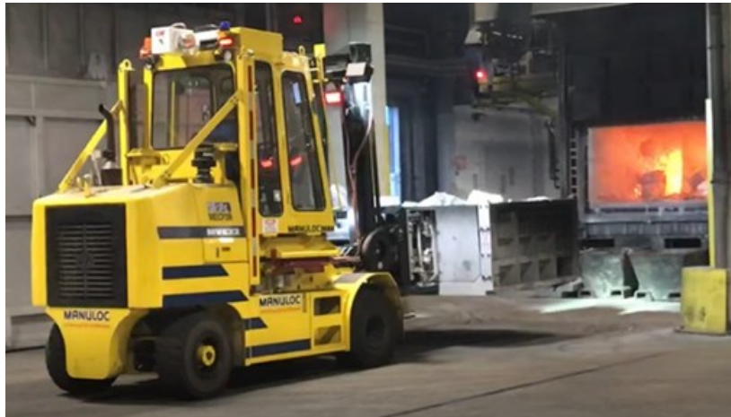
Figure 6. MVR22 carrying a pre-loaded bin of scrap.
