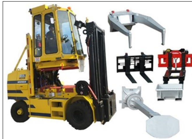
Figure 7. MVR - lifting cab with array of tools.
