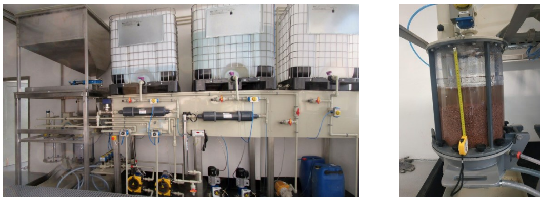
Figure 9. Extraction unit of the SPL-CYCLE pilot plant (left) and filled extractor during SPL processing (right).
