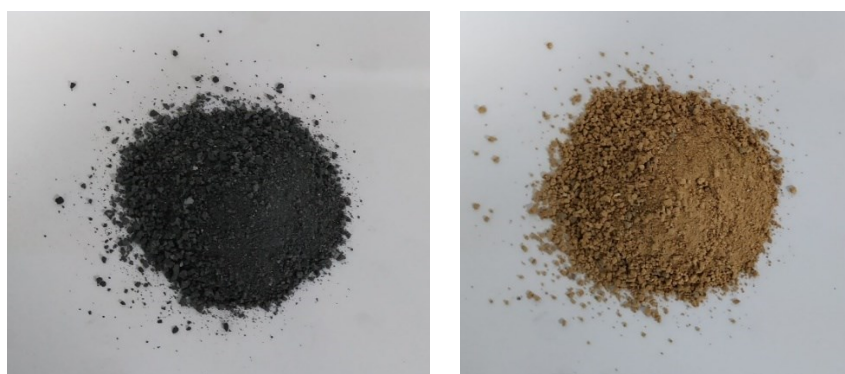
Figure 2. View of the SPL 1 st cut (left) and 2 nd cut (right).
