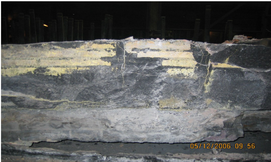
Figure 2. The “Lens” of interaction of infiltrated electrolyte and refractories: Top - schematic view of the cross-section; Bottom - cross-section of the cathode during the dry autopsy.
