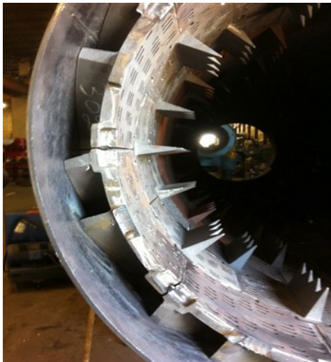
Figure 5. Liner interior flights.
