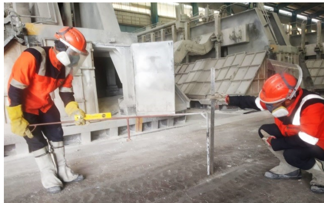
Figure 3. Metal/bath height measurement.
