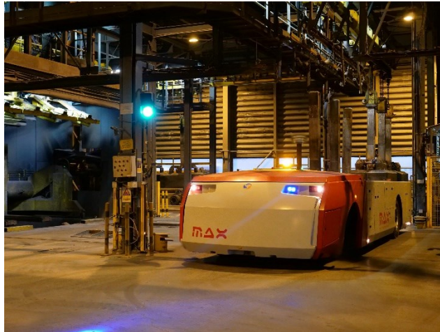
Figure 1. Anode transport vehicle (MAX) with full load of anodes.
