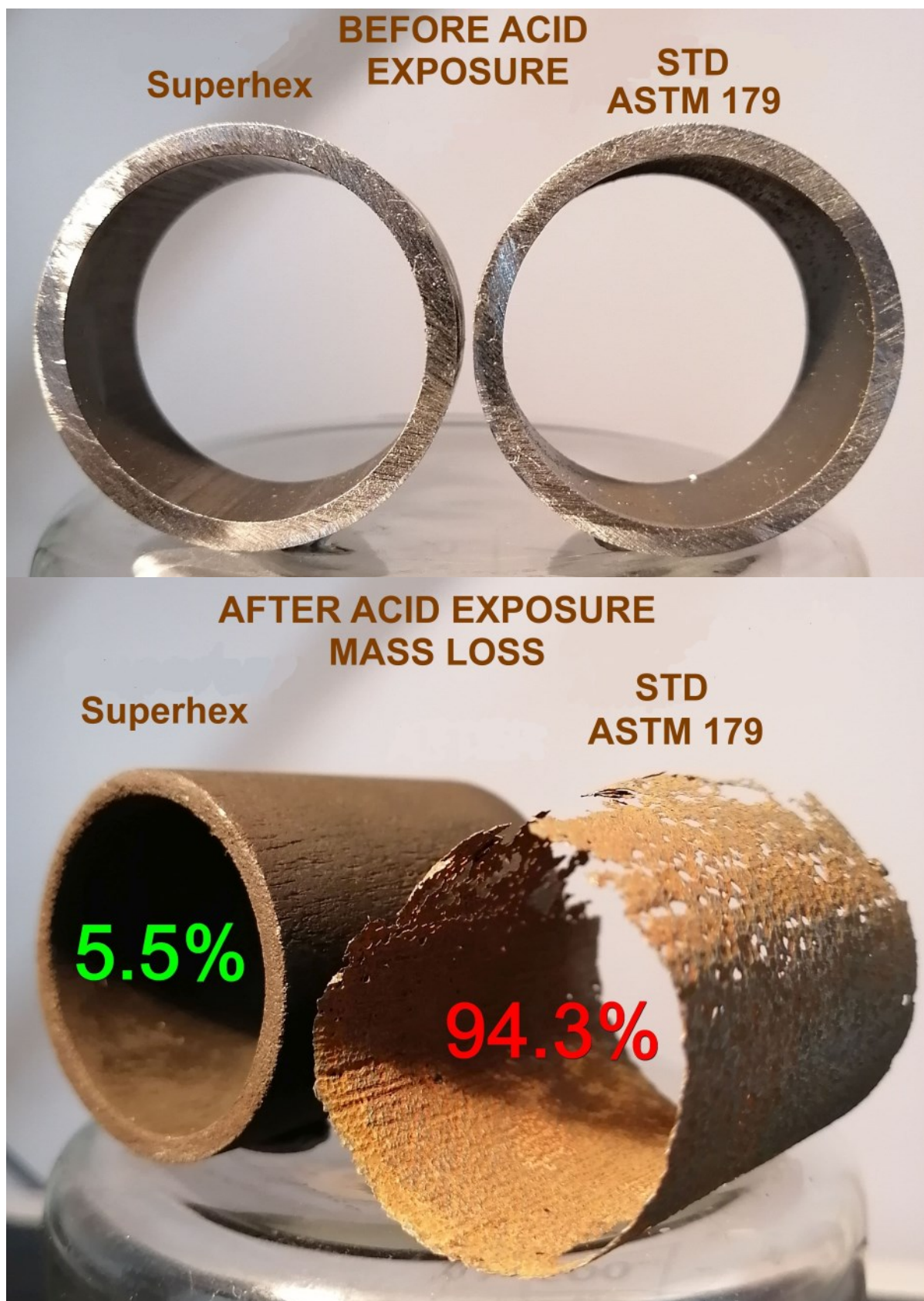
Figure 1. Mass loss images of Superhex vs STD ASTM 179.
