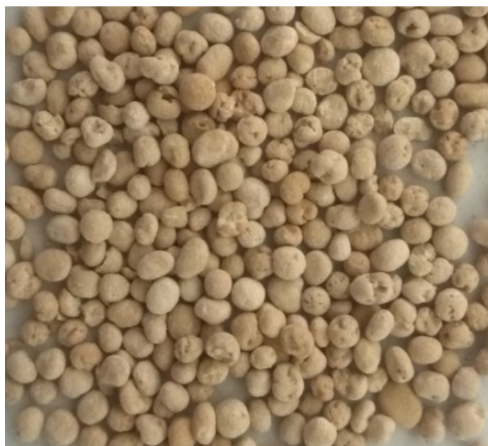
Figure 1. Sodium oxalate particles precipitated from diasporic digestion process.
