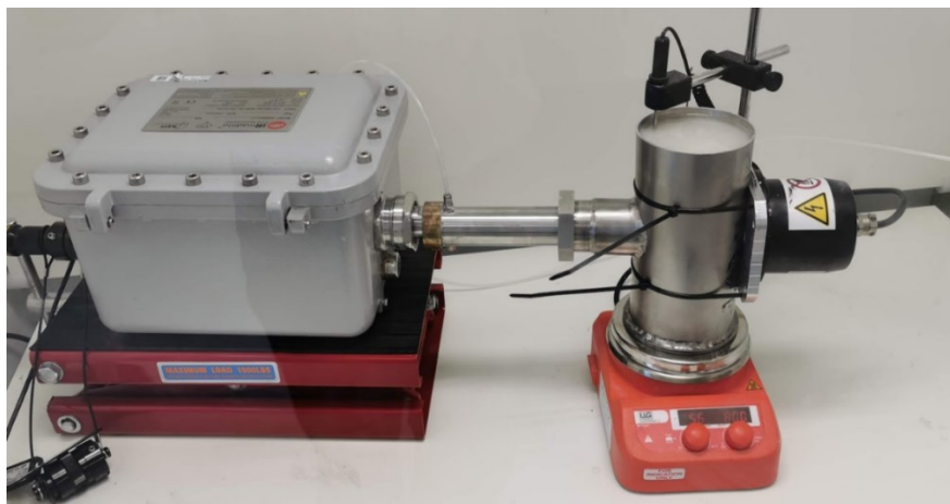
Figure 8. Photograph of the IRmadillo spectrometer installed into a sample cell with gibbsite scaling solution and an externally mounted ultrasonic transducer for descaling experiments.
