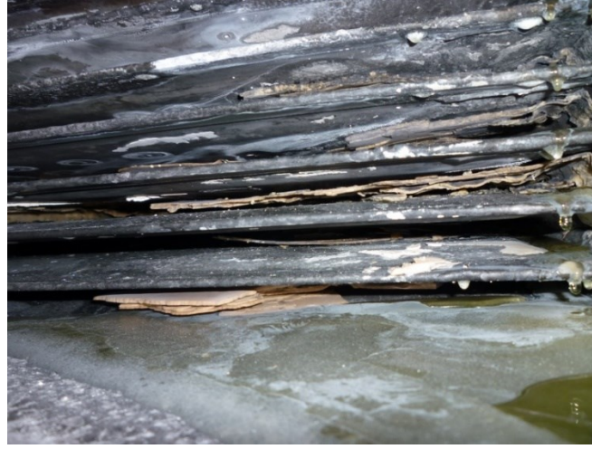
Figure 1. Scale on the heat transfer wall.
