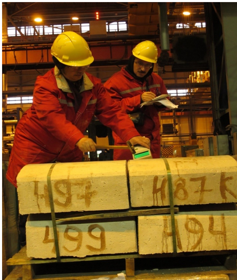
Figure 3. Control of large refractory blocks used in metallurgy, in process.
