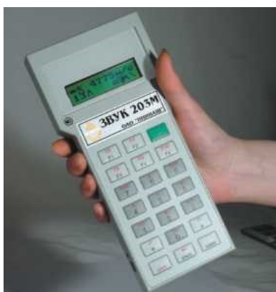
Figure 1. Device "Zvuk-203M" realize the free vibration method.
