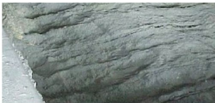
Figure 3. Wear of graphitized cathode blocks.
