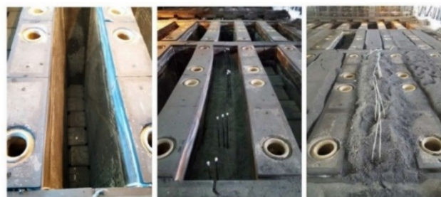
Figure 7. Procedure of imbedding thermocouples and protection pipes [1]
