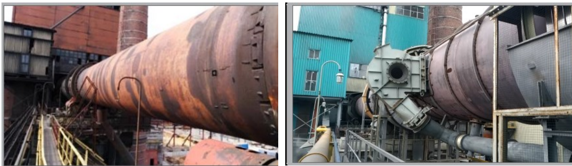
Figure 1. The coke calcining furnace. Left: before the retrofitting, right: after the retrofitting
