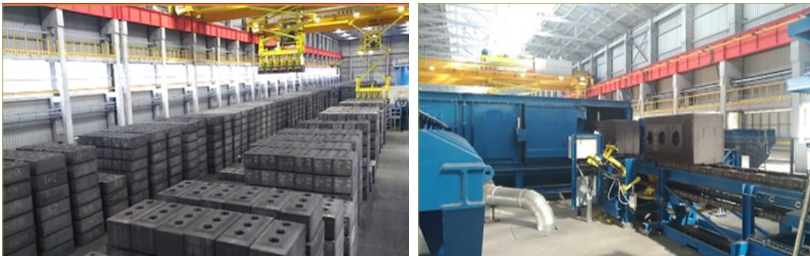
Figure 6. Left: a BA warehouse equipped with stacker cranes and a slot cutting machine, right: a BA conveyance line
