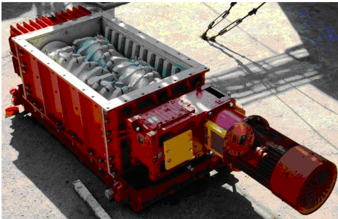
Figure 3. DShZ-500.20-75 (ДШЗ -500.20-75) double roll crusher with mining tooth.
