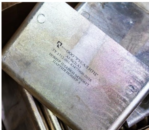
Figure 7. The photo of an Al-Sc master alloy produced by RUSAL as per GOST R 53777-2010.
