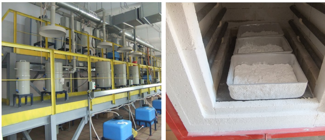
Figure 6. The pilot plant for the production of scandium oxide. Left: a scandium concentrate re-cleaning unit; right: a scandium oxide batch in the furnace.
