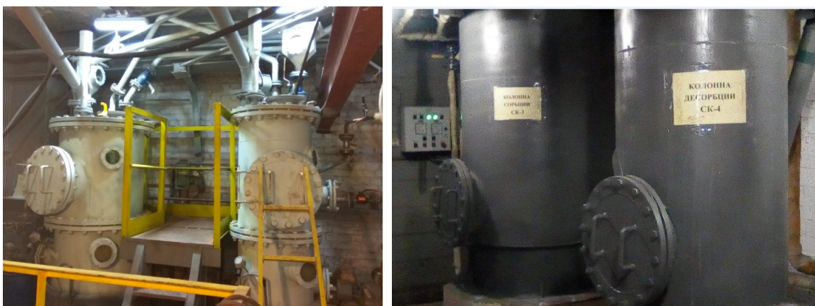
Figure 4. Photo showing a concentrating unit of scandium by sorption. Left: tops of the sorption and desorption columns; right: bottoms of the sorption and desorption columns.
