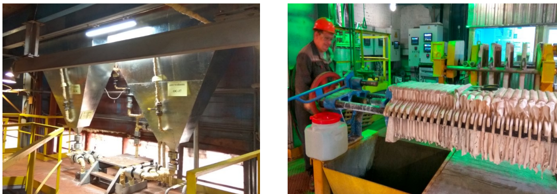
Figure 5. The photo showing the scandium concentrate extraction area. Left: precipitators for the preparation of scandium concentrate slurry before its filtration; right: filtration of scandium concentrate.
