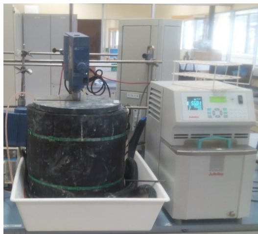
Figure 1. Laboratory unit for simulation of the process of bauxite residue lime neutralization.
