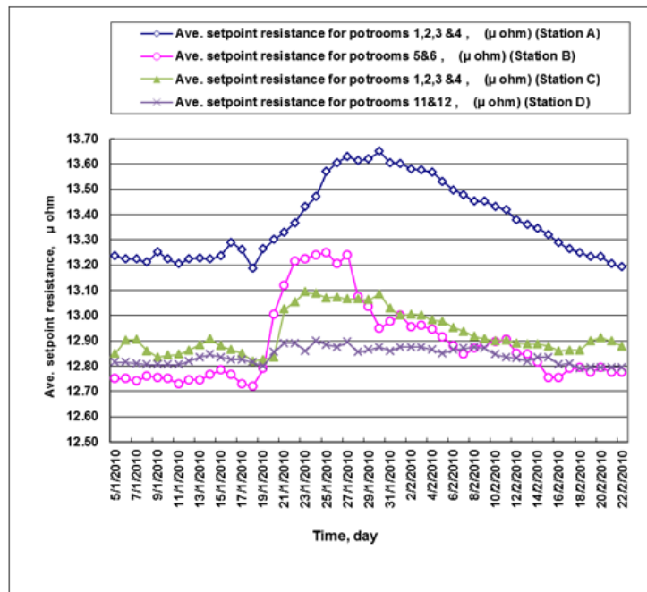
Figure 3. Variation in set-point resistance for power stations A, B, C and D (average values).
