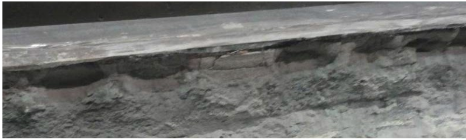
Figure 1. Example on severe degradation due to bad quality sidelining material. Plant A.
