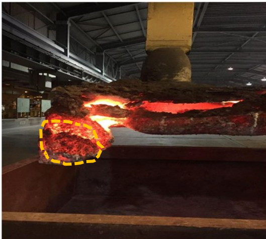
Figure 4. Extended anode spike.
