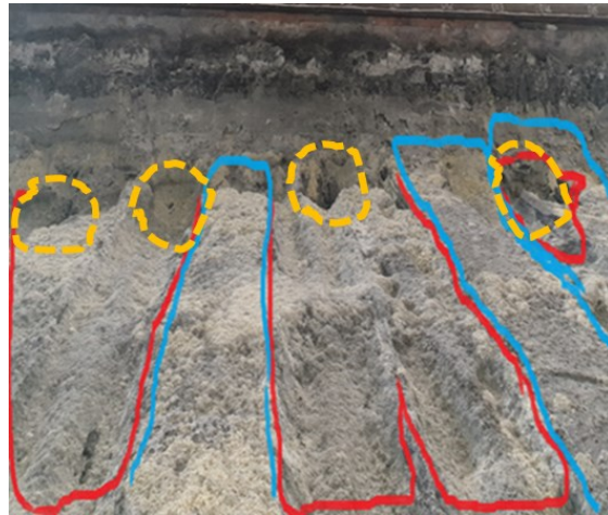
Figure 5. Deep-seated potholes in a graphitized cathode.
