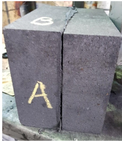
Figure 4. Vertical spreading on small slabs.
