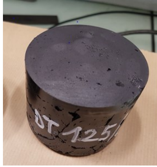
Figure 9. Aspect of 50 mm diameter sample of AD20+ after curing and sawing.
