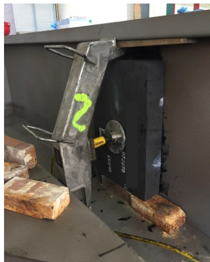
Figure 10. Model of a corner of a pot with AD20+ between the shell and graphite slab
