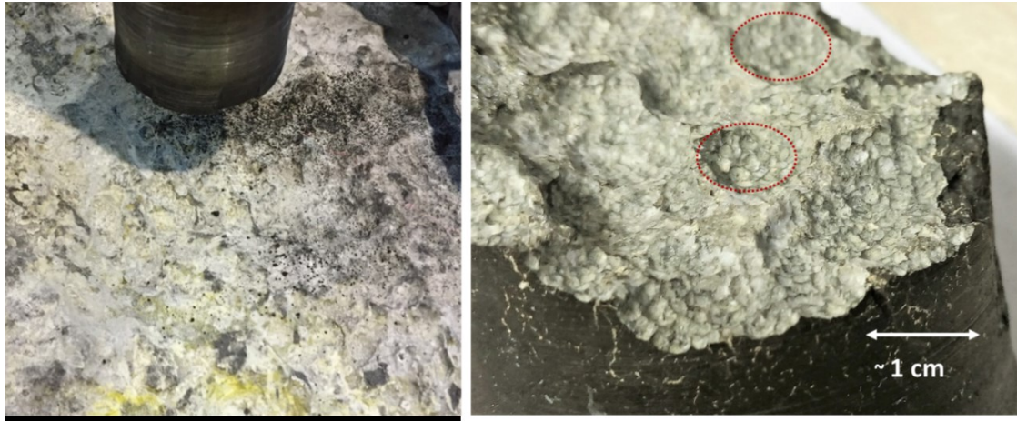
Figure 42 shows pictures of the cathode surface with pitting corrosion in one of the potholes located towards the outer ends of a cathode block.
