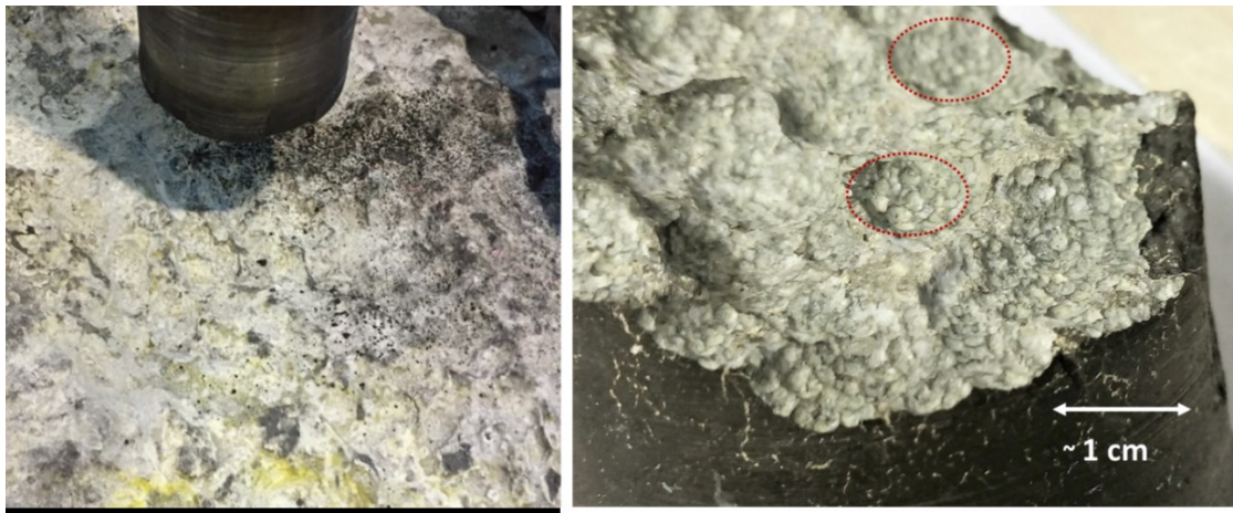
Figure 42. Pitting on the cathode surface of a spent potlining. Left picture includes part of the 5 cm diameter drill used to take core samples. Right picture shows more details of the micro wear pattern.
