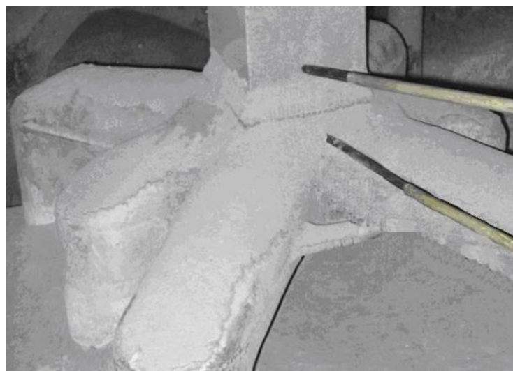
Figure 7. Position of probes while measuring the 'rod–yoke' voltage drop.
