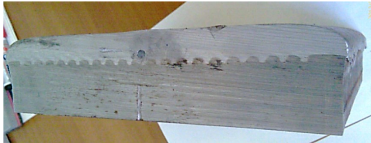
Figure 5. Bimetallic plate, type 2 with titanium interlayer.
