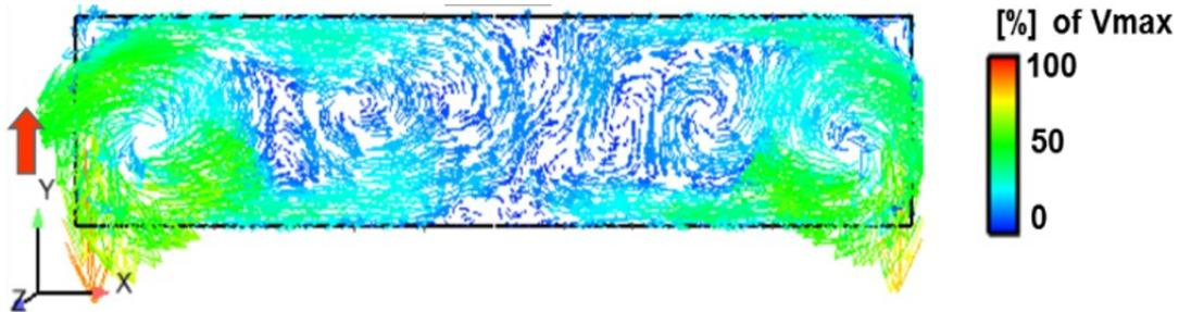
Figure 10. Velocity field in a pot calculated with Alucell.
