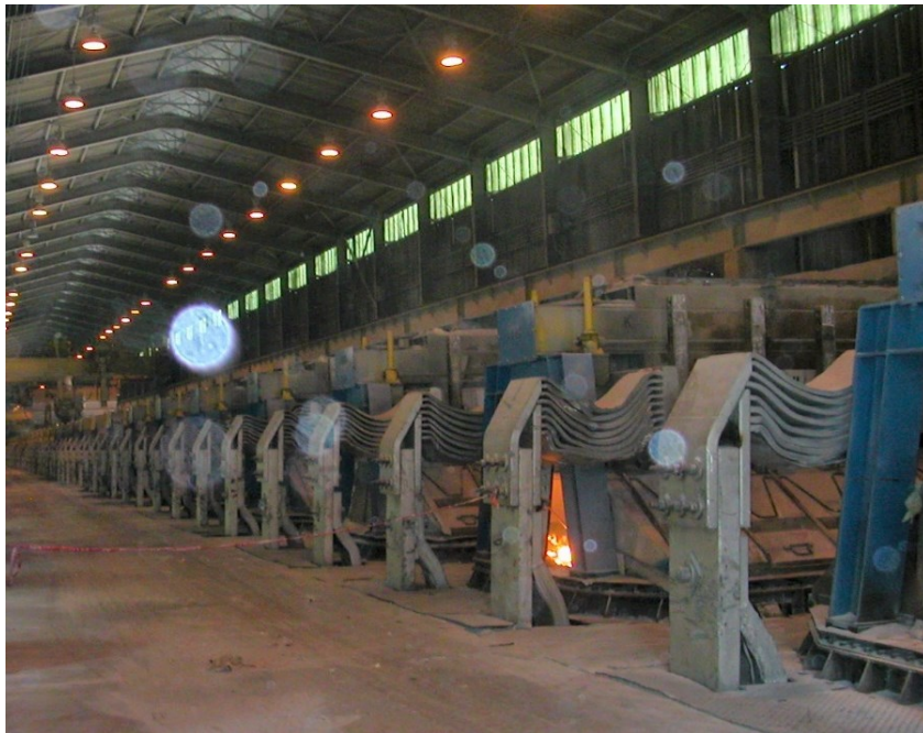
Figure 25. Reynolds P-19 line at Valesul smelter (shutdown in 2009, currently dismantled).
