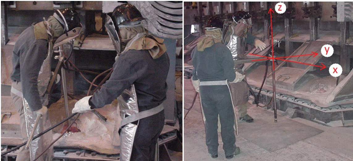
Figure 37. Left: Measurements being performed inside the metal pad by CAETE staff employing the magnetic probe. Right: Probe coordinate system.
