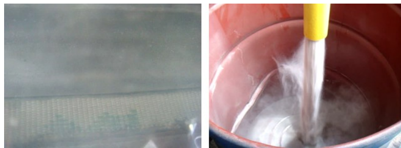
Figure 10. Test rig of a 76.2 mm internal diameter, 9.3 m long round air slide at [6].
