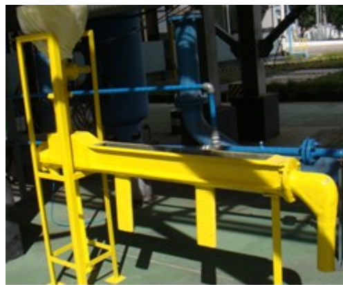
Figure 8. Air-fluidized conveyor of 1.5 m long with three outlets [6].
