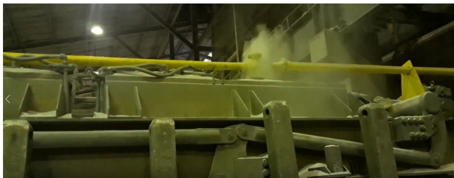
Figure 13. Dust emission on Pot 239 during the alumina feeding process.
