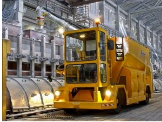
Figure 3. Pot superstructure alumina hopper filling with a truck [2].
