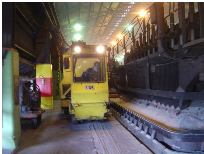
Figure 2. Alumina feeding by truck to the side of a Søderberg pot [1].
