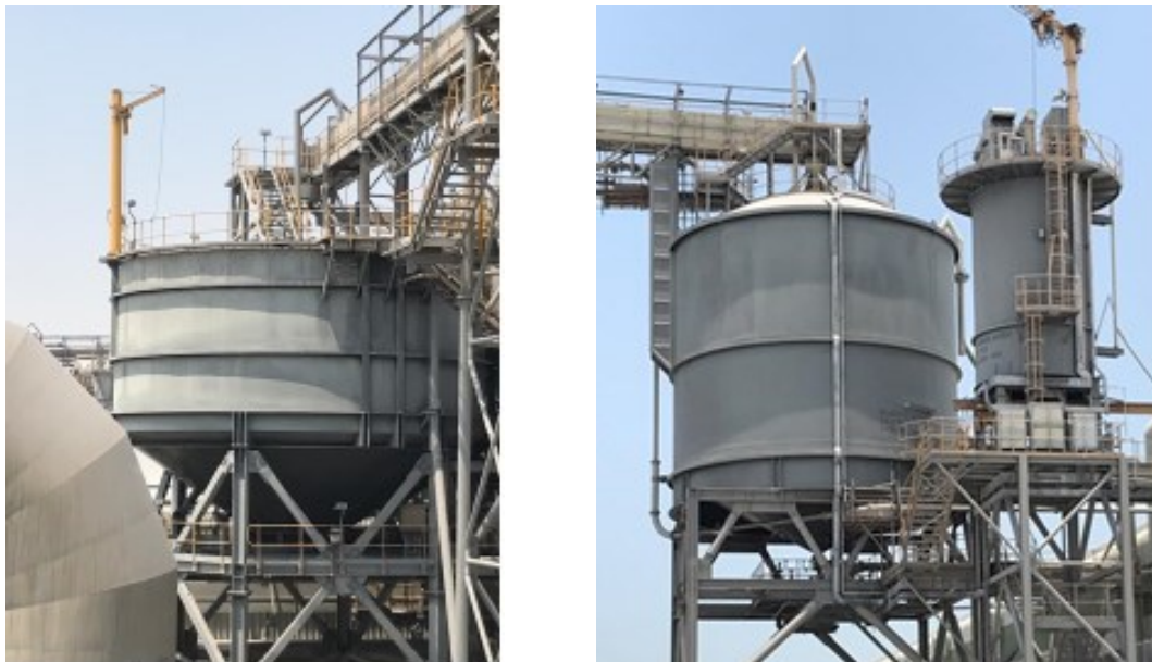
Figure 8. Left: EGA Al Taweelah Phase 1 low aspect ratio enriched alumina silo driven by height constraints and Right: EGA Al Taweelah Phase 2 standard aspect ratio enriched alumina silo, both with anti-segregation systems on top.
