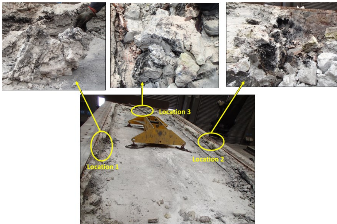
Figure 2. Ledge sampling locations in the cell, Location 3 is at the DUCT END.
