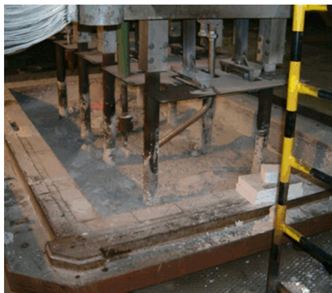
Figure 8. Alumina top cover on the experimental 25 kA cell.
