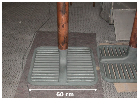
Figure 2. Example of NILO anode tested in a 25 kA cell [4].
