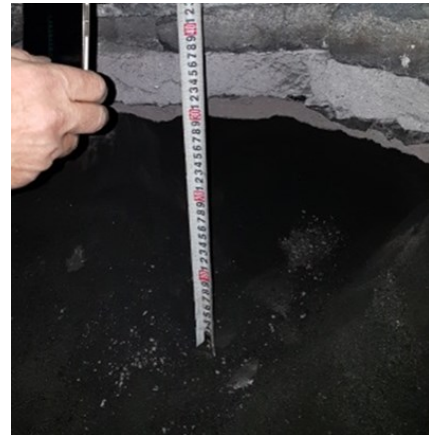
Figure 7. Cross section with lignite semi-coke in the free state.
