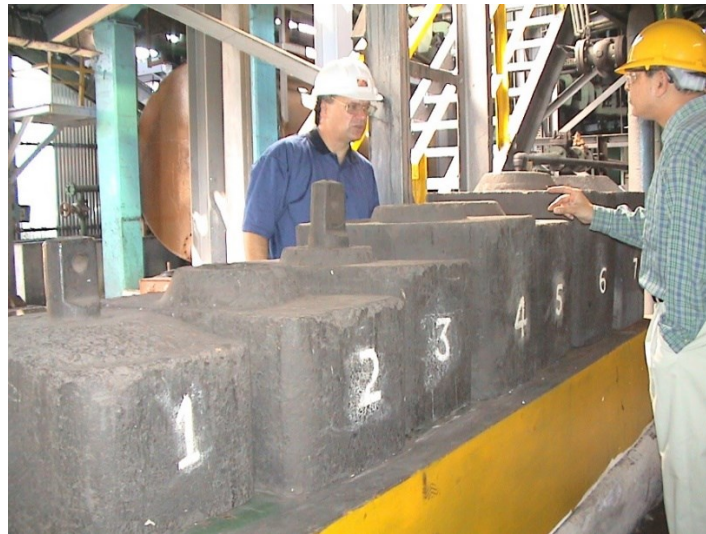
Figure 1. Illustration of the change in anode sizes (from 1 to 7) used in cells originally designed for 55 kA to enable line current increase.
